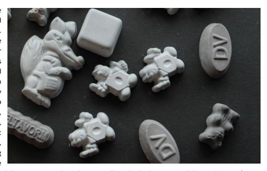
don't have the model's digital data, we scan it three dimensionally and edit the generated data with our software. Then, we send the digital data to our MDX-540. The machine takes care of the rest."
